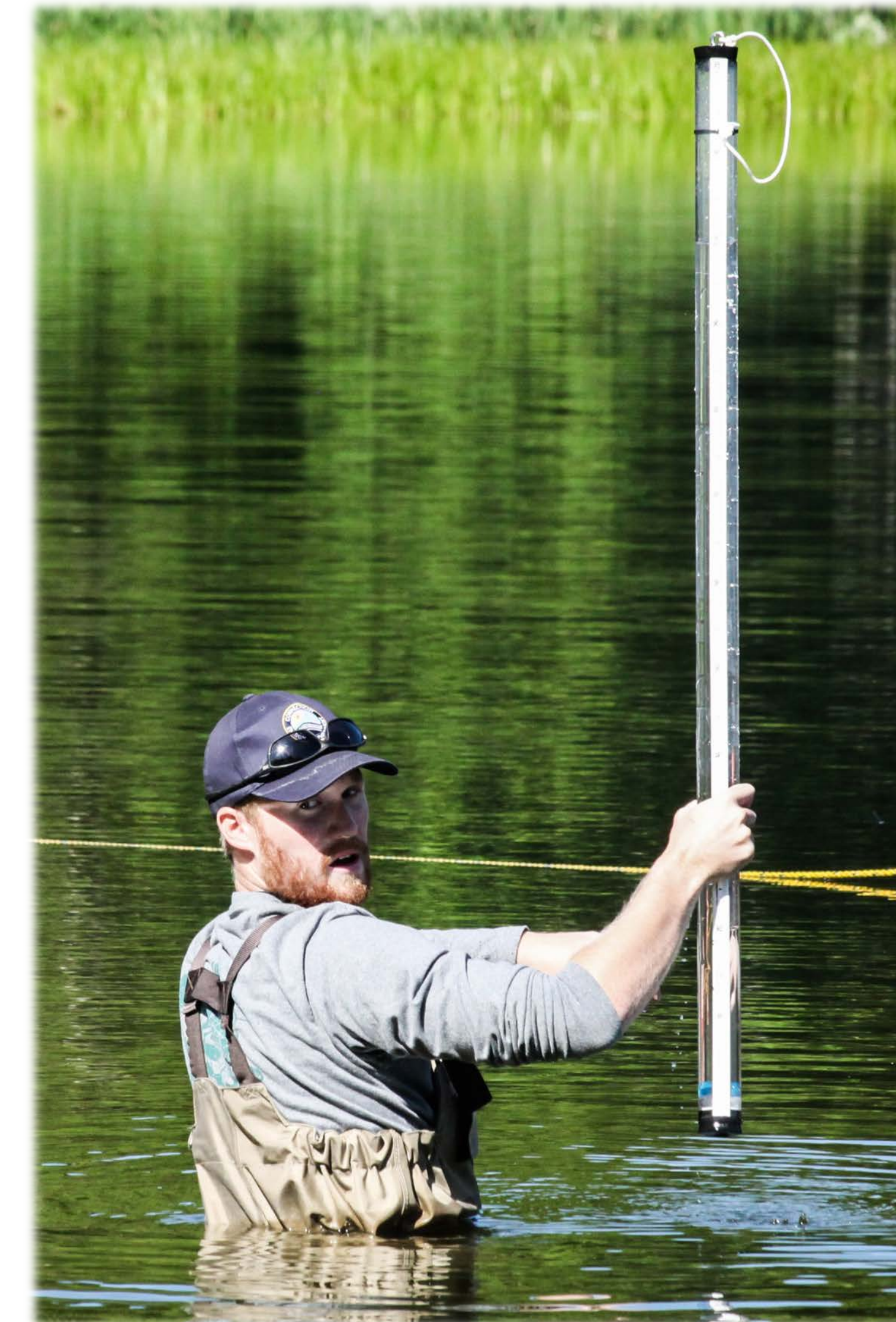
Figure 2. Sampling Mount Tom Pond State Park with integrated water sampling tube.
