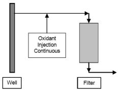
Manganese Greensand Process with Continuous Regeneration
