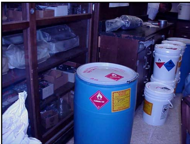
Figure 7 - Chemicals are packed into 5 gallon pails or 55 gallon drums. The drums are then sent off for recycling, fuels blending, or secure landfilling.
