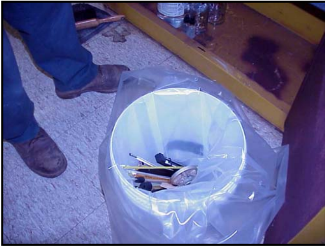
Figure 5 - Mercury containing lab instruments are placed into a lined container meeting all Department of Transportation requirements
