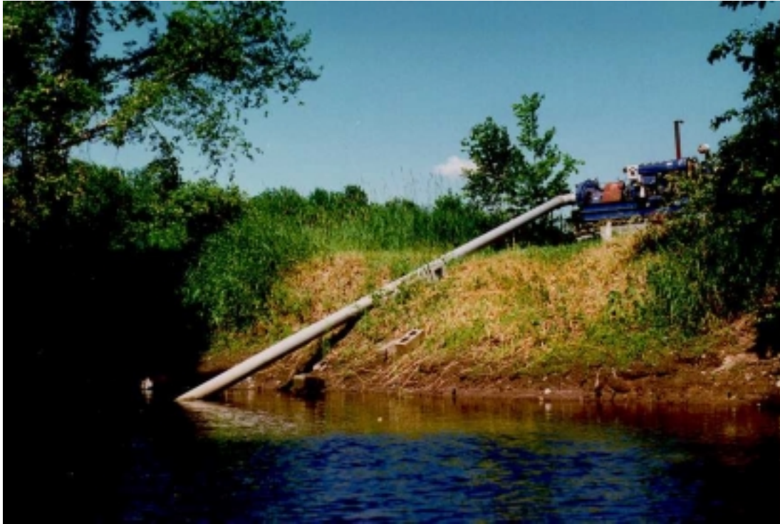
Tractor-mounted pump with pipeline to the river, used for an agricultural diversion, Quinnipiac River
