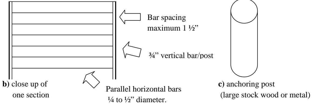
*Note – Parallel bars can be secured to 3/4" vertical bars 48" apart or attached directly to large stock anchoring posts.*
