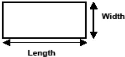
$$\text{Surface Acreage} = \frac{\text{width in ft} \times \text{length in ft}}{43,560 \text{ sq. feet}}$$
